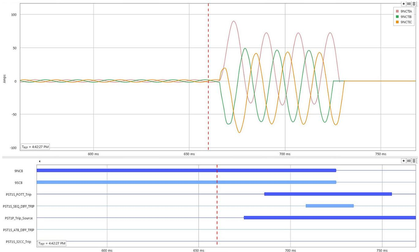
Fig. 15. Three-Phase Internal Fault at FLOC 1 Tap Neutral
