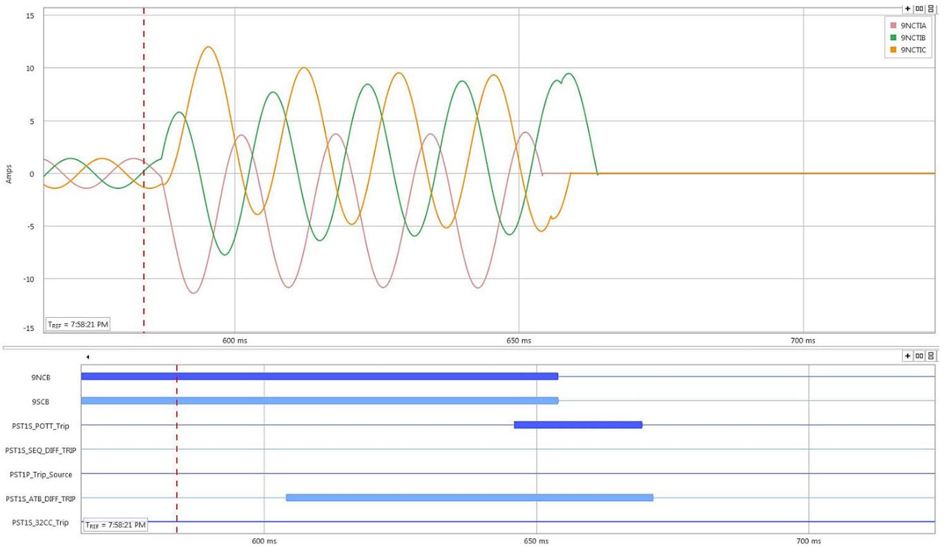
Fig. 17. Three-Phase Internal Fault at FLOC 2 Tap R10
