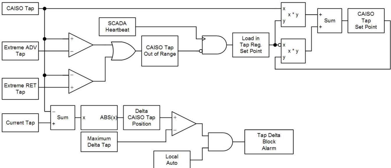
Fig. 10. PST Controller Tap Position Control Logic
