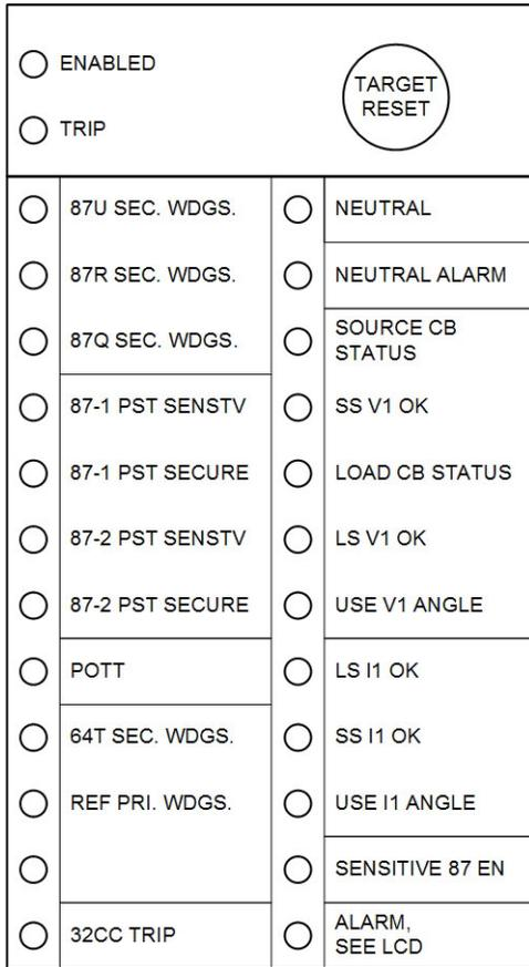
Fig. 8. 87S and 87O Relay PST Protection Front Panel
