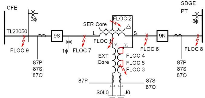
Fig. 14. System One-Line Diagram and Tap Position Control Logic
