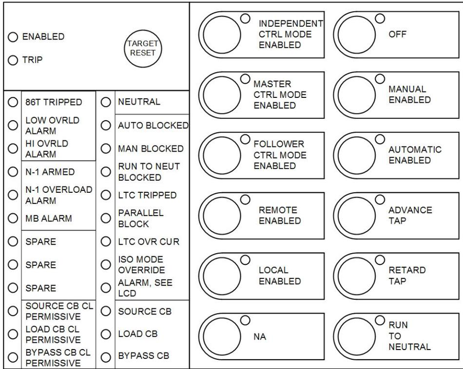
Fig. 9. PST Controller Front Panel
