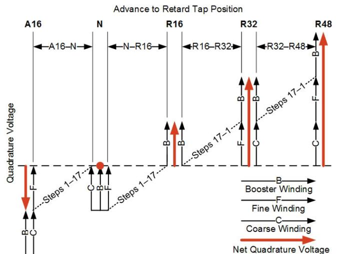
Fig. 3. Three Secondary Windings Provide Wide Range of Regulation
