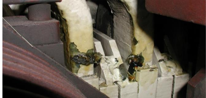
Fig. 1. Damage caused by a neutral-side fault.
