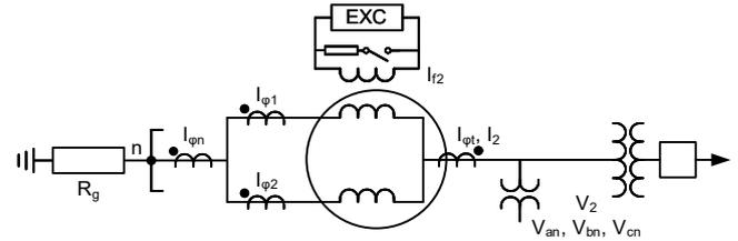
Fig. 7. Single-line diagram with instrument transformer signals used by protection functions.
