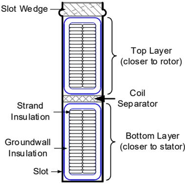
Fig. 5. Machine with Roebel bars on two layers separated by a Bakelite separator.
