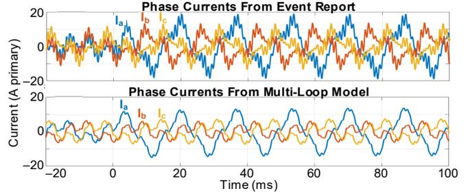
Fig. 3. Response comparison between the scale-model machine (top) and the simulation (bottom) for a five-turn interturn fault.
