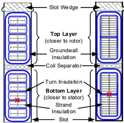
Fig. 6. Possible interturn fault locations in the slot for a machine with a form-wound multi-turn coil (left) or a two-turn Roebel bar (right).
