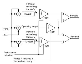
Fig. 1. Simplified logic of the TD32 element for the Phase-A-to-ground (AG) loop.
