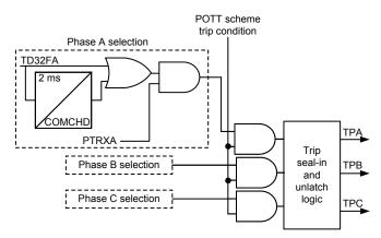
Fig. 5. Phase selection and trip logic for the POTT scheme.
