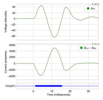
Fig. 9. Incremental voltage and replica current of the CG loop captured at MID and the TD32 protection element operation for the internal fault on May 4.
