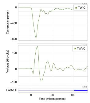
Fig. 8. TW current and voltage captured at MID and the TW32 protection element operation for the internal fault on May 4.
