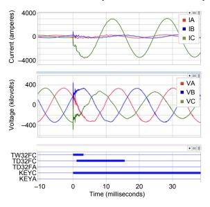
Fig. 6. Currents and voltages captured at MID and the timedomain protection element operation for the internal fault on May 4.
