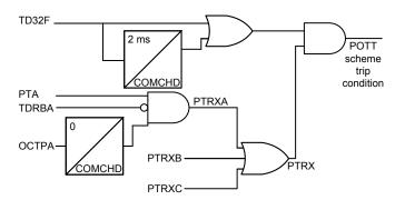
Fig. 4. Receiver logic provides security to the POTT scheme.
