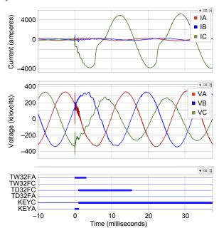
Fig. 7. Currents and voltages captured at TMD and the time-domain protection element operation for the internal fault on May 4.
