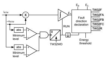
Fig. 2. Simplified logic of the TW32 element.
