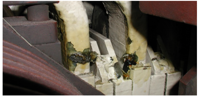
Fig. 1. Damage caused by a neutral-side fault.
