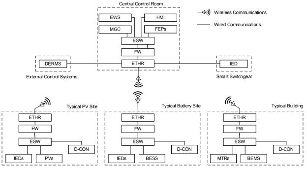
Fig. 4. Overall MGCS network architecture
