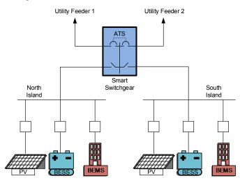
Fig. 2. Simplified one-line diagram of proposed microgrid
