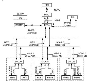
Fig. 5. Communications data flow diagram
