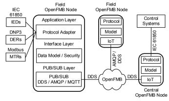
Fig. 6. Example OpenFMB framework model
