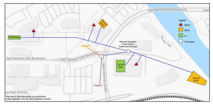
Fig. 1. Microgrid power system overview map
