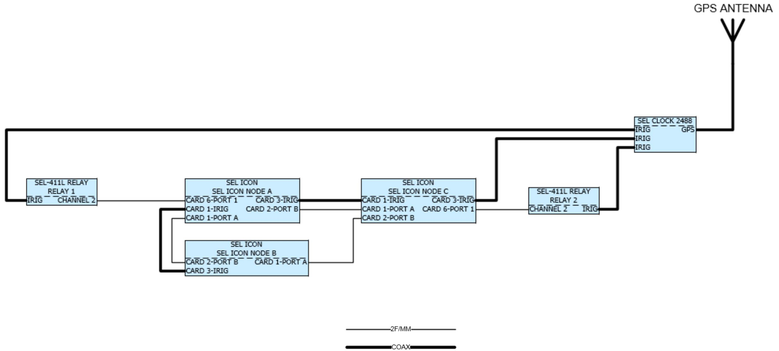
Figure 6-3 – ICON Baseline Test Setup
