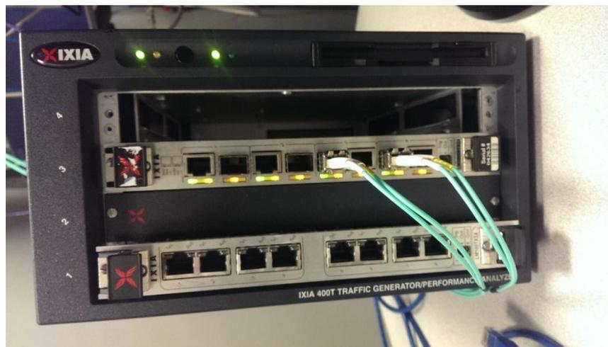
**Figure 4-1 – IXIA Network Traffic Generator**
