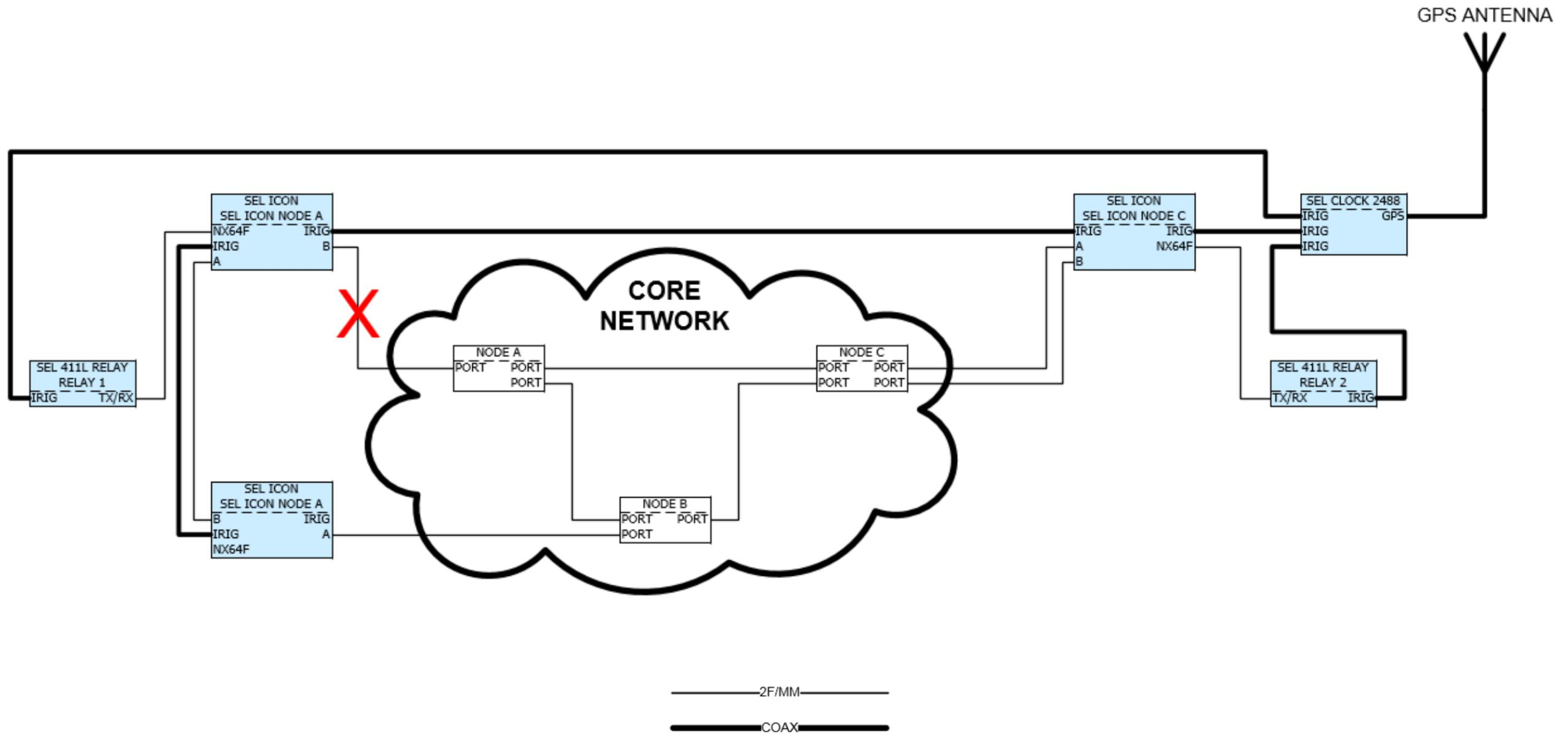
Figure 6-11 – ICON Failover Test Setup
