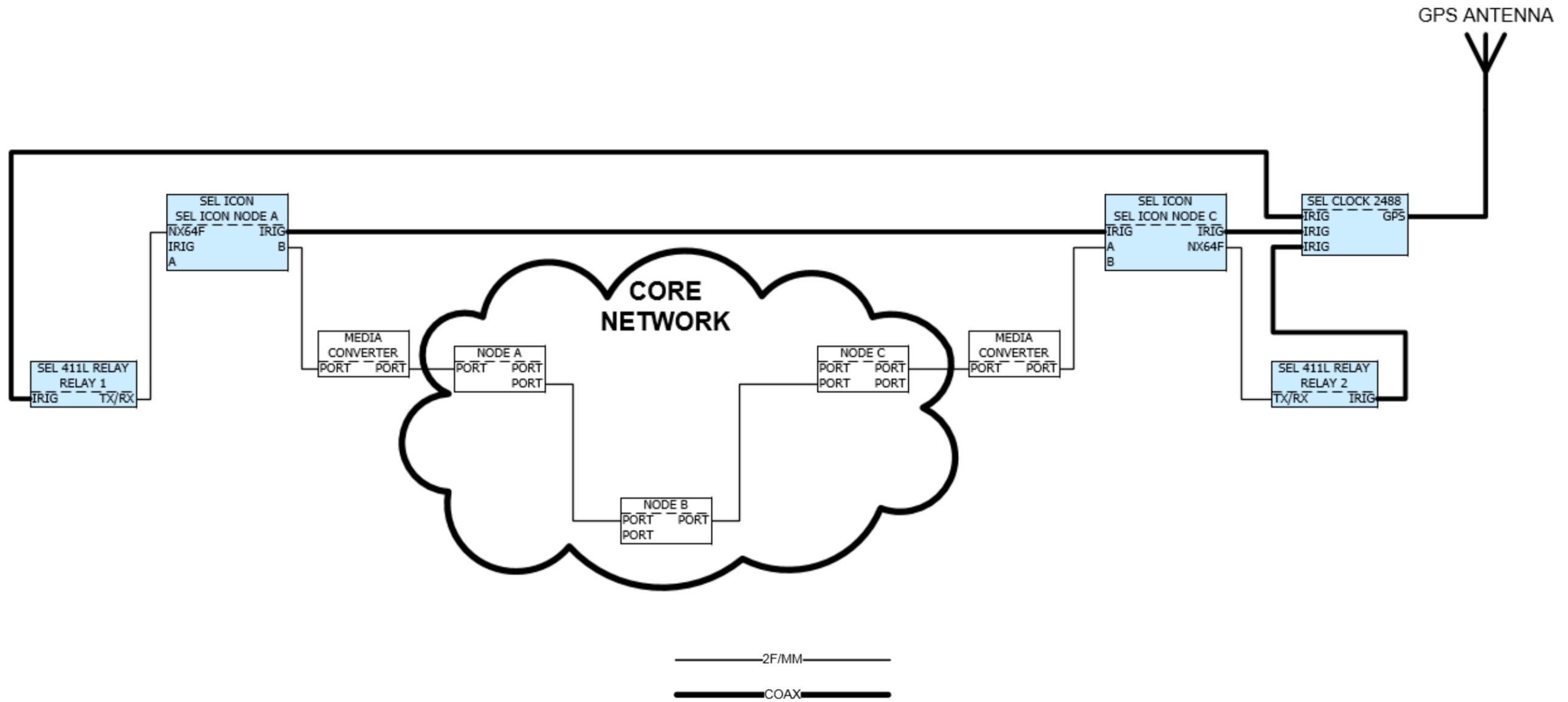
Figure 6-7 – ICON/Cisco Network Baseline Test Setup
