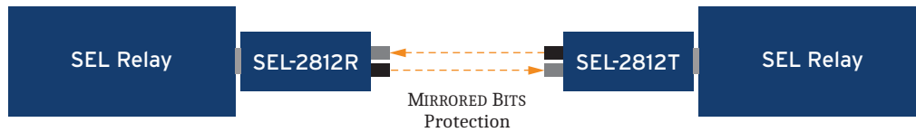
Figure 3 MIRRORED BITS Communications Example
