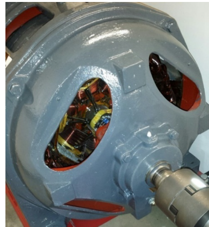
Fig. 5. 18 kVA, 6-pole machine used for multi-loop model
