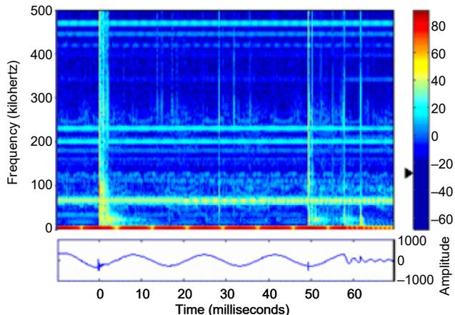
Fig. 22. Phase C (faulted phase) voltage waveform frequency content evolution over time.
