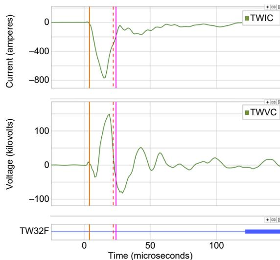
Fig. 24. TW phase current and voltage are of opposite polarities. Therefore, TW32 declared the event as forward.
