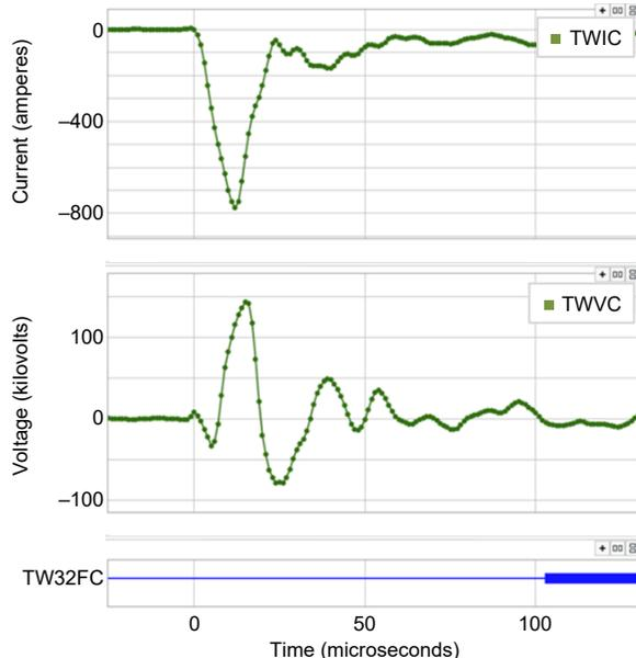
Fig. 28. TW current and voltage captured at MID and the TW32 protection element operation for the internal fault on May 4.
