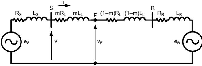
Fig. 2. Two-source single-phase system with a fault at F.
