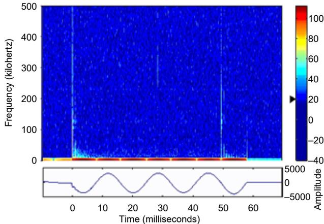
Fig. 21. Phase C (faulted phase) current waveform frequency content evolution over time.
