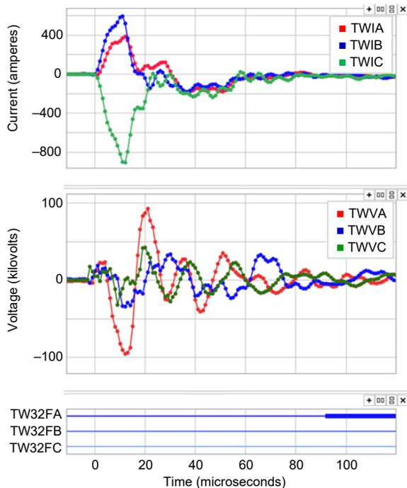
Fig. 29. TW currents and voltages captured at TMD and the TW32 protection element operation for the internal fault on May 4.
