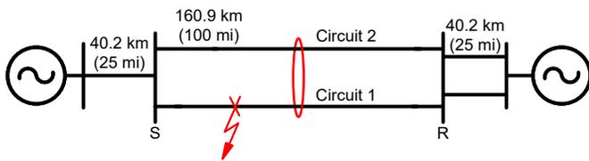
Fig. 11. An AG fault simulated on Circuit 1.
