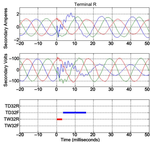
Fig. 14. The TW directional element declared the fault shown in Fig. 11 as reverse at Terminal R.
