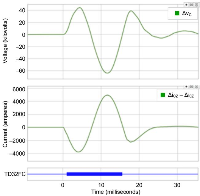
Fig. 30. Incremental voltage and replica current of the CG loop captured at MID and the TD32 protection element operation for the internal fault on May 4.
