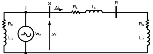
Fig. 4. Fault network of the Fig. 2 system for a fault behind Terminal S (a reverse fault for a relay at Terminal S).
