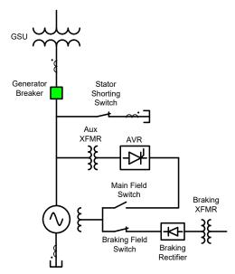
Fig. 15. Typical Configuration of a Dynamic Braking Setup for a Reversible PSH Unit
