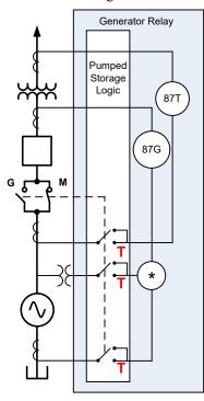
Fig. 6. Relay With Integrated Pumped Storage Logic
