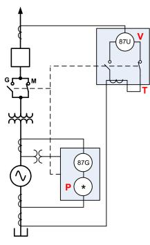
Fig. 10. Reversing Switch Upstream of the GSU
