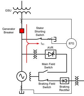
Fig. 17. Shorting Switch Applying a System Fault
