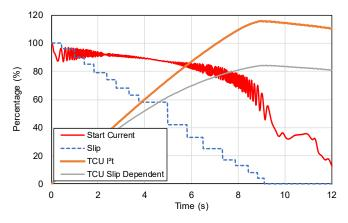
Fig. 9. Slip-Dependent vs I<sup>2</sup>t Thermal Model
