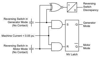
Fig. 7. Operating Mode Logic
