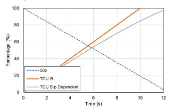
Fig. 8. Slip-Dependent vs l<sup>2</sup>t Thermal Model Assuming Constant Current Magnitude
