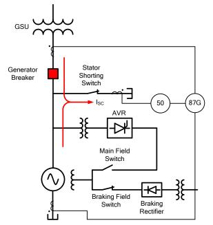
Fig. 18. Dynamic Braking Overcurrent Protection
