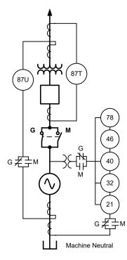
Fig. 2. E/M Relays and CT/PT Secondary Switching
