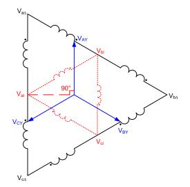
Fig. 11. Reduced-Voltage Starting Using Three Midwinding Taps
