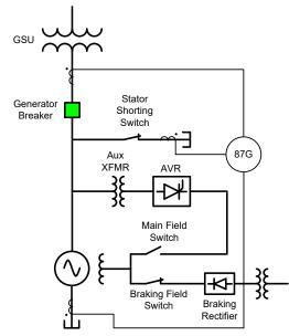
Fig. 16. Dynamic Braking Differential Protection (Dynamic Braking Equipment Not Shown for Clarity)
