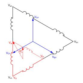
Fig. 12. Reduced-Voltage Starting Using Two Midwinding Taps
