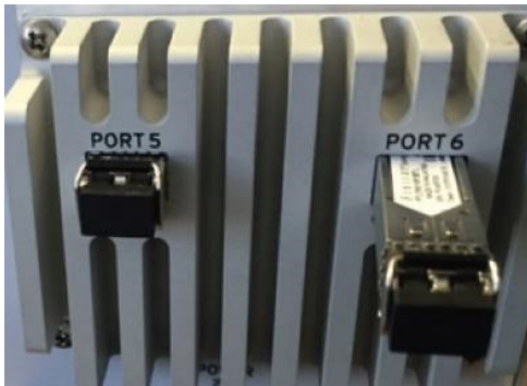
Fig. 2. SFP transceiver installation example
