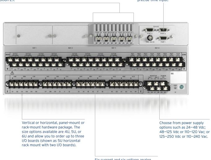
Six current and six voltage analog inputs, orderable in standard terminal blocks (shown) or a Connectorized® hardware configuration.
