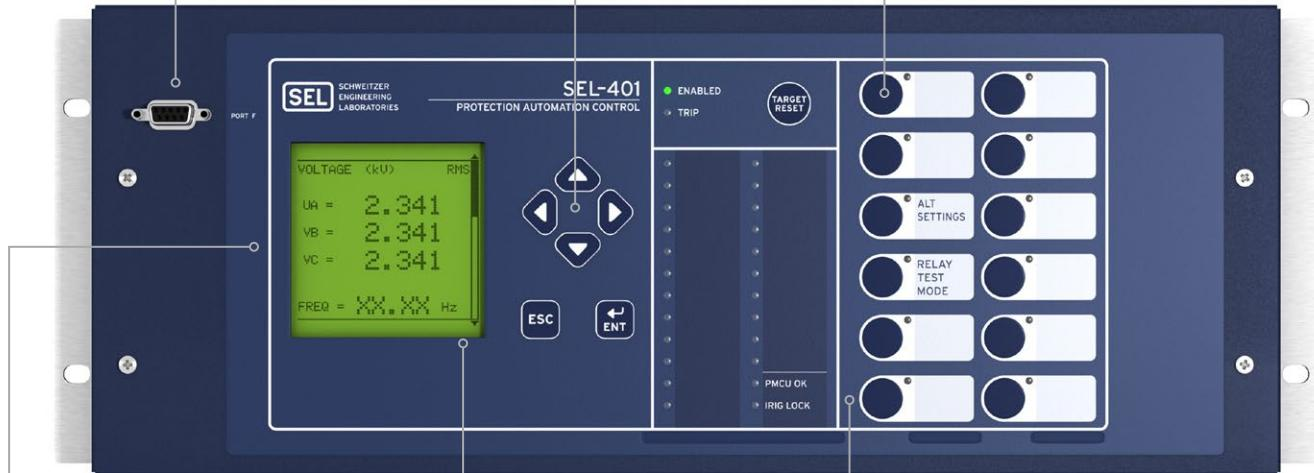
The front-panel display provides status indication and control of as many as ten disconnects. The merging unit offers control for up to two breakers and provides status indication for up to three breakers.
