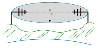
Fig. 5. Fresnel Zone Between Antennas
