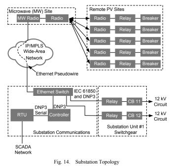
Previous projects with similar communication via DERs used MIRRORED BITS communications serial protocol to send transfer trips to the PV system breakers and used DNP3 protocol to bring back statuses, watts, and VARs. MIRRORED BITS communications is a fast serial protocol that is limited to two interfaces per relay. Because of this limitation, IEC 61850 GOOSE was selected for its ability to scale up the number of interfaces for the remote sites. DNP3 was maintained for SCADA.
