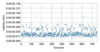
Fig. 17. Round-Trip Latency With GOOSE Messages Every 20 ms and No DNP3
