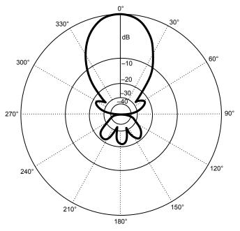
Fig. 10. Directional Yagi Antenna Radiation Pattern
