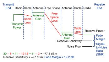
Fig. 12. Example of an End-to-End Link Budget
