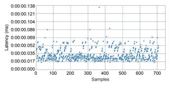
Fig. 16. Round-Trip Latency With GOOSE Messages Every 20 ms and DNP3
