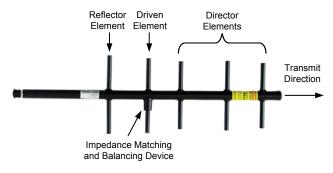
Fig. 9. Directional Yagi Antenna
