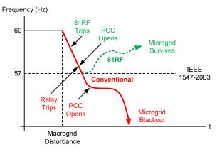
Fig. 7. Proactive Automatic Islanding Before a Microgrid Blackout
