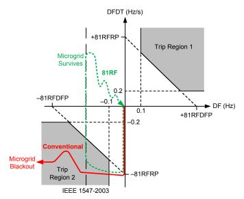
Fig. 6. 81RF Element Assists Microgrid Survival
