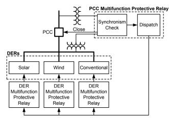
Fig. 2. Multifunction Relays Performing PCC A25A Function
