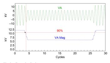
Fig. 2. Example of voltage sag
