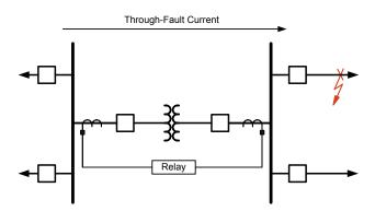
Fig. 6. One-line diagram of a typical through fault event
