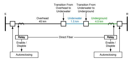
Fig. 7. TWFL in a real-world hybrid transmission line
