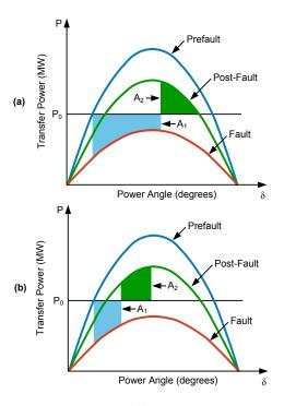
Fig. 5. Power system transfer capability and the equal-area criteria in (a) an unstable system and (b) a stable system
