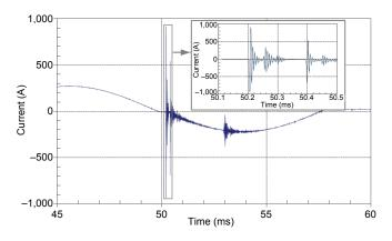
Fig. 10. Current reignition (60 Hz system)
