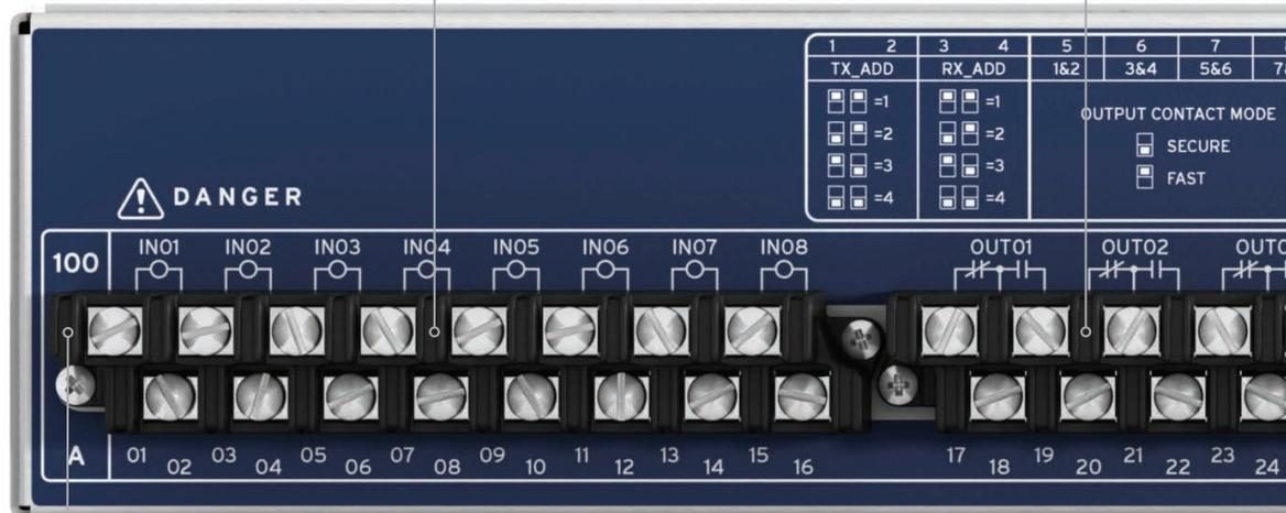
Connectorized screw terminals accept ring lugs with wires up to #10 AWG.
