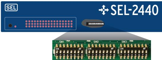
**SET PROTOCOL AND ADDRESS USING DIP SWITCHES**
