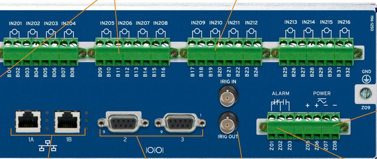
Standard 10/100BASE-T Ethernet ports with integrated switch eliminate the need for an external switch.
