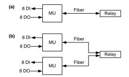
Fig. 6. Connections for a point-to-point system with a single I/O connection (a) and multiple I/O connections (b)
