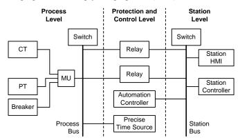
Fig. 2. Substation configuration with a station bus and process bus
