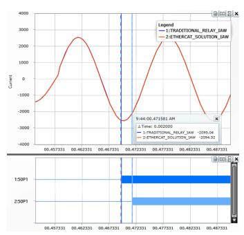
Fig. 8. Performance of a traditional relay and an EtherCAT-based relay
