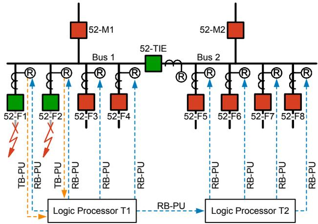
Fig. 10. Double-Circuit Feeder Trip Scheme
