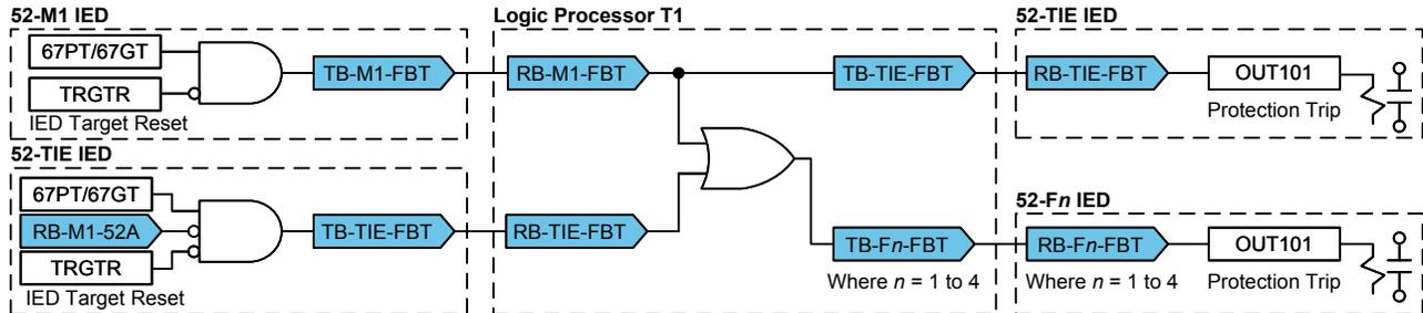
Fig. 6. Fast Bus Tripping Logic Diagram
