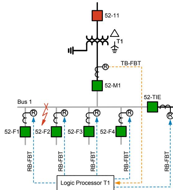
Fig. 4. Fast Bus Tripping Scheme
