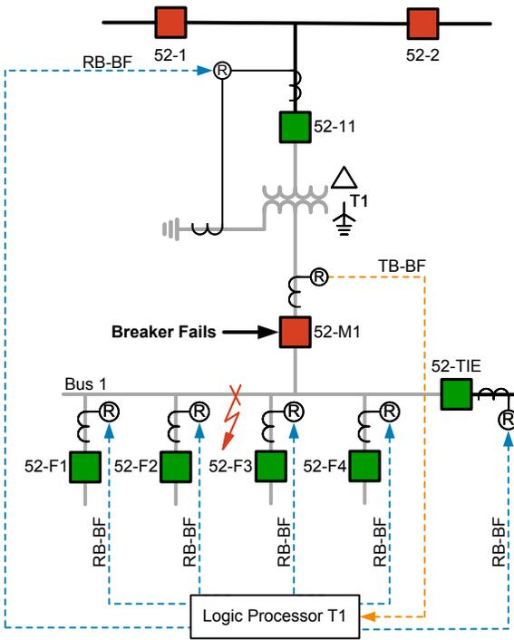
Fig. 8. Breaker Failure Protection Scheme
