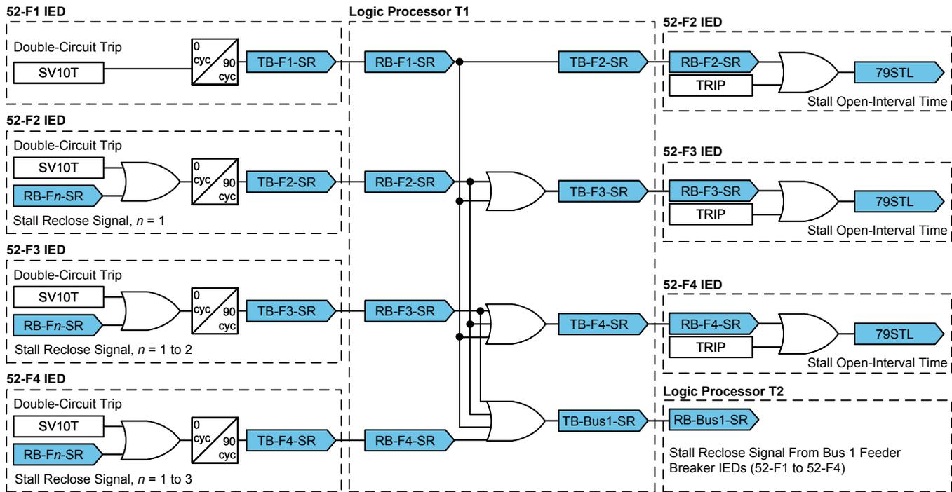
Fig. 12. Stall Reclose Logic Diagram
