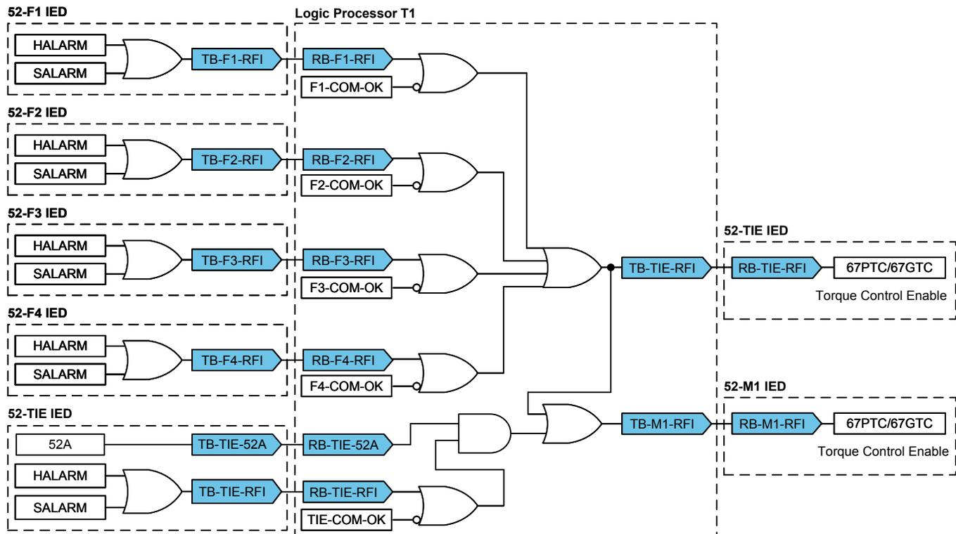
Fig. 15. IED Failure Initiate Scheme Logic Diagram
