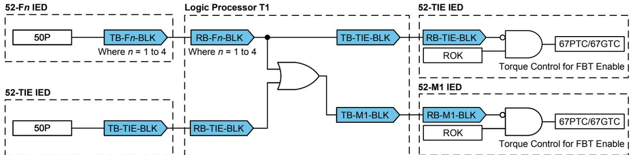
Fig. 7. Fast Bus Tripping Block Logic Diagram
