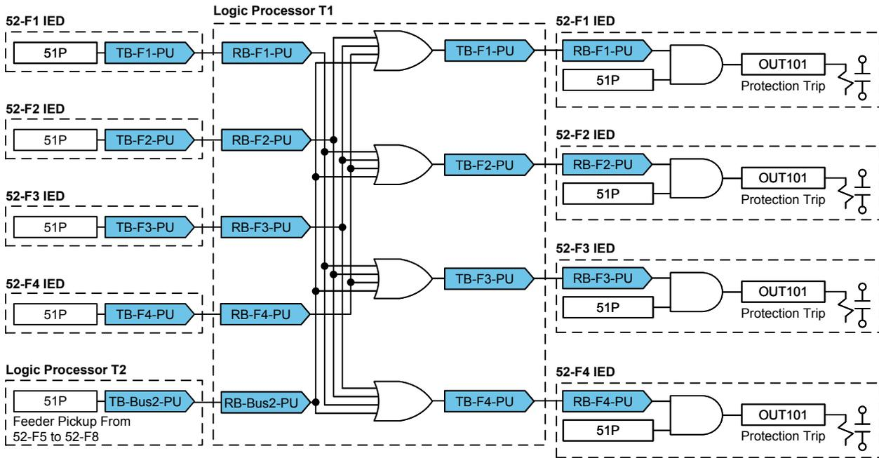
Fig. 11. Double-Circuit Feeder Trip Logic Diagram
