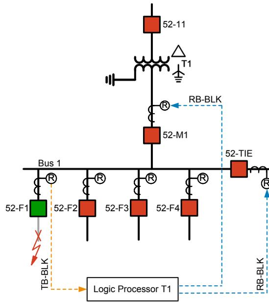
Fig. 5. Fast Bus Tripping Block
