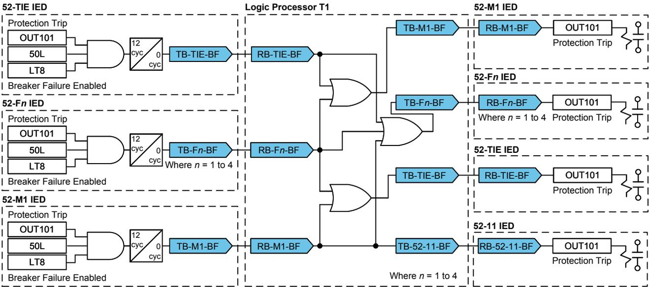
Fig. 9. Breaker Failure Protection Logic Diagram
