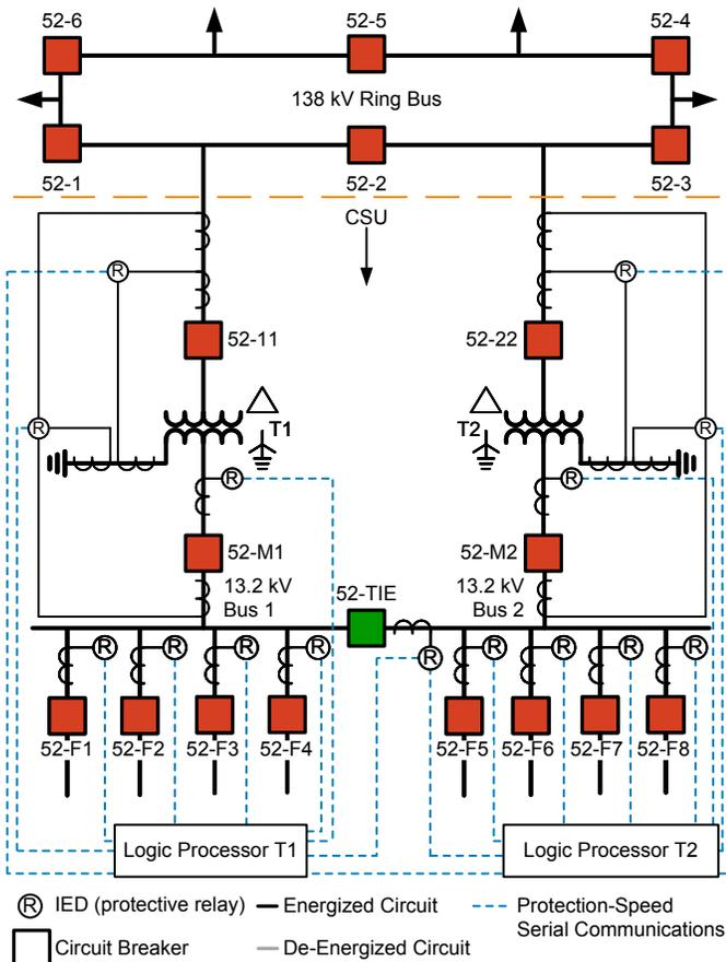
Fig. 1. Simplified One-Line Diagram for a Typical COCS Distribution Substation (the key applies to all one-line diagrams in this paper)
