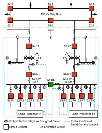
Fig. 1. Simplified One-Line Diagram for a Typical COCS Distribution Substation (the key applies to all one-line diagrams in this paper)
