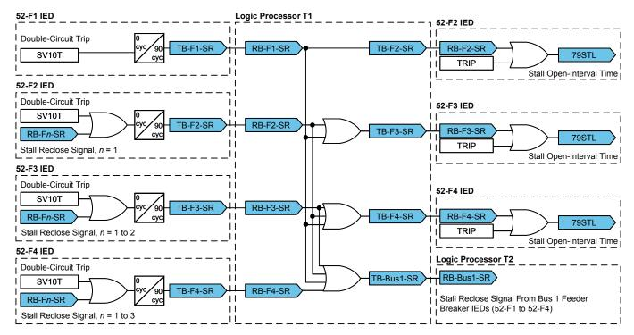
Fig. 12. Stall Reclose Logic Diagram
