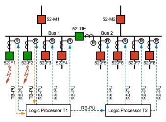
Fig. 10. Double-Circuit Feeder Trip Scheme
