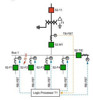
Fig. 4. Fast Bus Tripping Scheme
