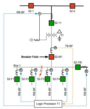
Fig. 8. Breaker Failure Protection Scheme
