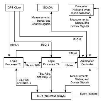
Fig. 3. Information Flow Diagram for a Distribution Substation
