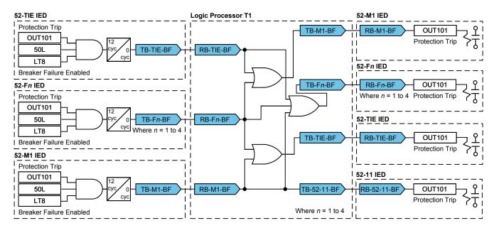
Fig. 9. Breaker Failure Protection Logic Diagram
