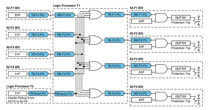
Fig. 11. Double-Circuit Feeder Trip Logic Diagram
