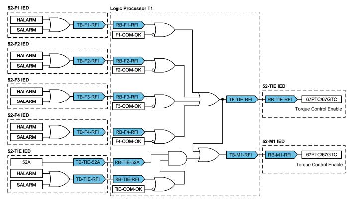
Fig. 15. IED Failure Initiate Scheme Logic Diagram
