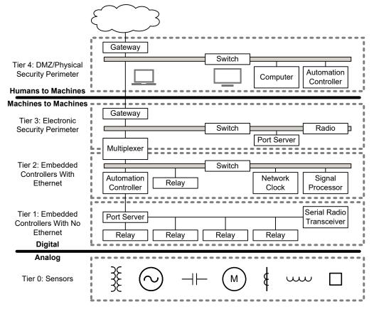
Figure 2 Substation Security Model
