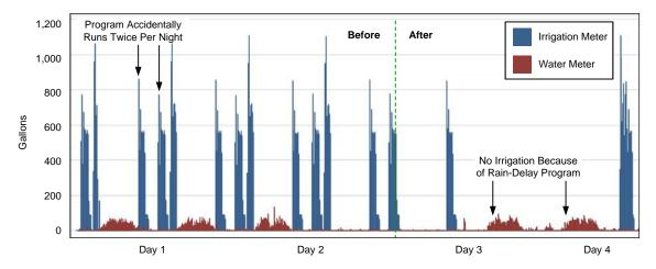
Figure 3—Trend of Water Consumption Before and After Change in Irrigation Program
