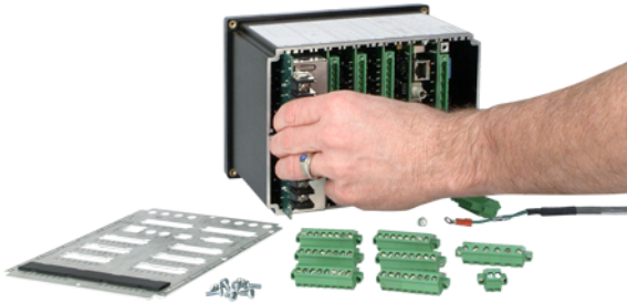
Detach connectors. Remove rear cover.
