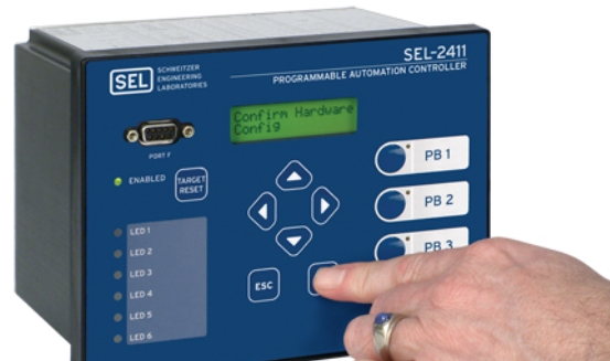
Energize and accept new I/O configuration.
