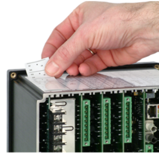
Install cards. Install new I/O labels on top of chassis.
