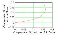
Fig. 2. Bus S compensated ground loop impedance ( $k_0 = 0.66 \angle 0^\circ$ ).
