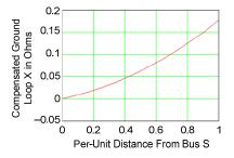
Fig. 5. Bus S compensated ground loop reactance ( $k_0 = 0.66 \angle 0^\circ$ ).
