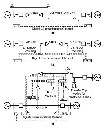
Fig. 9. Mixed overhead and underground circuits.
