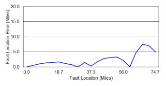
Fig. 31. Manufacturer B SLG impedance-based fault locator
