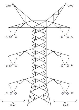
Fig. 4. Tower configuration for the 500 kV and 230 kV lines
