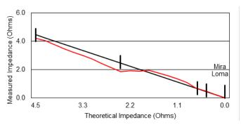
Fig. 17. Mira Loma terminal three-phase impedance measurement of Manufacturer A
