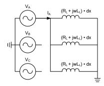
Fig. 15. Zero-sequence impedance test connection
