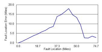
Fig. 32. Manufacturer B 3LG impedance-based fault locator
