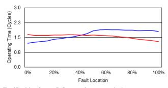
Fig. 27. Manufacturer B distance relay average trip times
