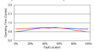
Fig. 26. Manufacturer A distance relay average trip times
