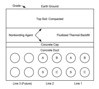
Fig. 8. Concrete duct bank
