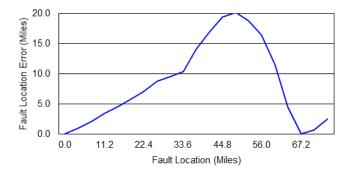
Fig. 30. Manufacturer A 3LG impedance-based fault locator
