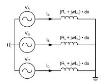
Fig. 14. Positive-sequence impedance test connection
