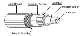
Fig. 7. XLPE cable construction
