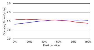
Fig. 28. Manufacturer B current differential relay average trip times
