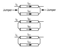
Fig. 5. Jumpered phase conductors
