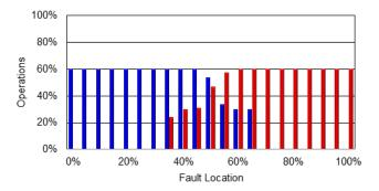
Fig. 24. Manufacturer A ground instantaneous overcurrent elements
