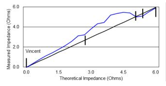
Fig. 16. Vincent terminal three-phase impedance measurement of Manufacturer A
