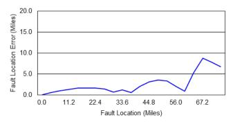
Fig. 29. Manufacturer A SLG impedance-based fault locator
