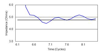
Fig. 21. Manufacturer A mho ground impedance measurement
