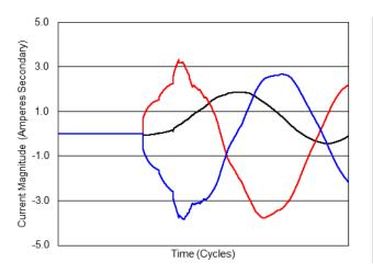
Fig. 34. Secondary currents injected into the relay
