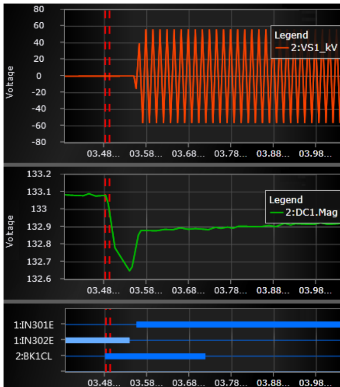
Fig. 3. Bus Energization Test Bus Voltage, Trip Bus Voltage, and Trip/Close Statuses
