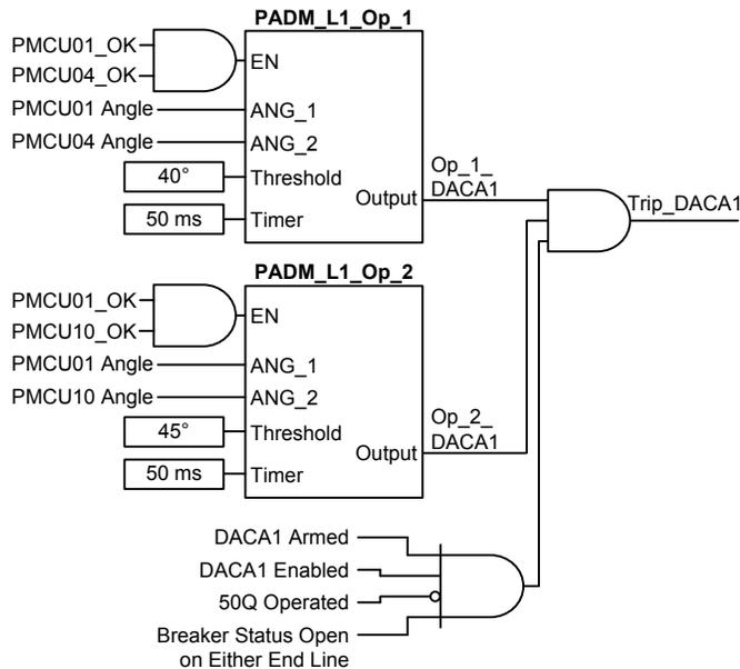
Fig. 10. PADM logic diagram to send trip command
