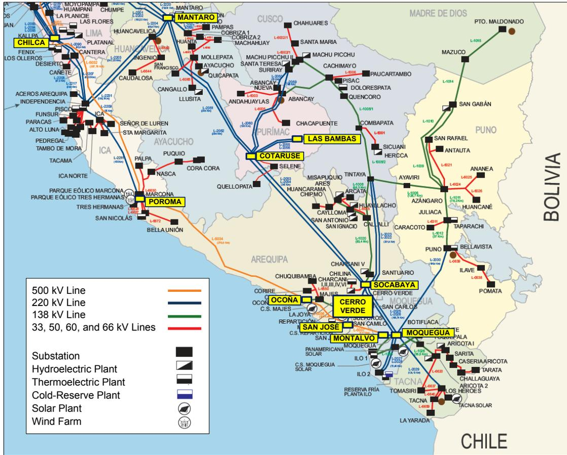
Fig. 1. Geographical view of the 500 kV (orange) and 220 kV (blue) lines
