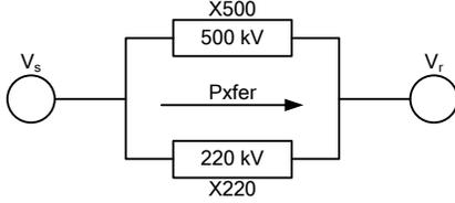
Fig. 3. Simplified representation of the Peruvian power system
