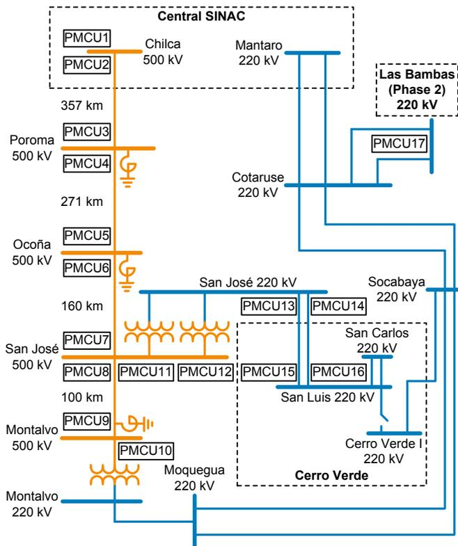
Fig. 2. Simplified representation of the components of the remedial action scheme (RAS)
