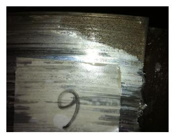
Fig. 17. Enlargement showing damage to white metal thrust bearing.
