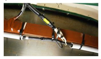
Fig. 22. A Rogowski coil with a test winding.
