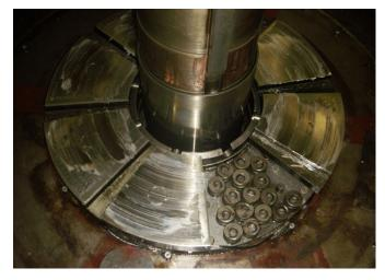
Fig. 16. Thrust bearing damage due to shaft currents (see striations in the bearing).
