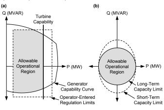
Fig. 2. Dynamic Capability Monitoring in a Typical Combustion Turbine Driven Generator (a) and a Typical Battery Storage System (b)
