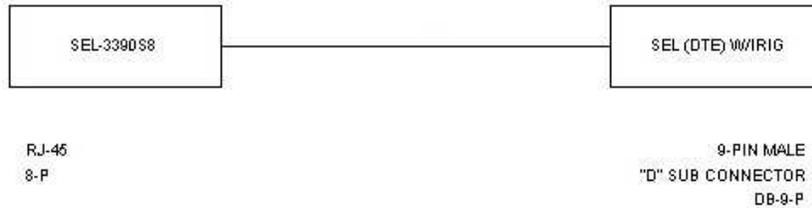
**CABLE:** 4 Pair (Stranded) Twisted Shielded Industrial Cat5E Cable
