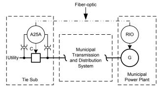
Fig. 3. Municipal microgrid with remote synchronizing.
