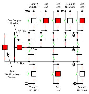
Fig. 6. Synchronizing with a complex switchable bus [8].
