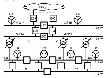
Fig. 1. Simplified one-line diagram of refinery power system [2].
