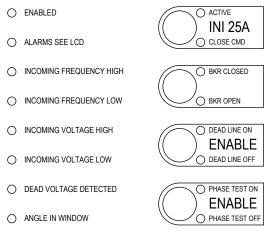
Fig. 5. Portable synchronizer controls and indications.
