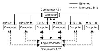
Fig. 1. Triple modular redundant supervisory architecture.
