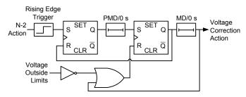
Fig. 6. Voltage correction logic.
