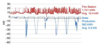
Fig. 2. Seven-Day Load Profile of FS24 and Solar Production
