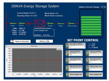
Fig. 8. Battery Monitoring Detail Screen
