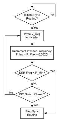
Fig. 6. Synchronization Routine Logical Diagram
