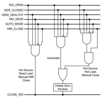
Fig. 5. Initiate Synchronization Routine Logic Algorithm
