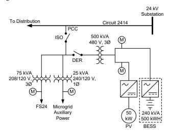
Fig. 3. Microgrid One-Line Diagram
