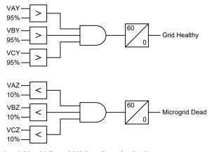
Fig. 4. Grid and Microgrid Voltage Detection Logic
