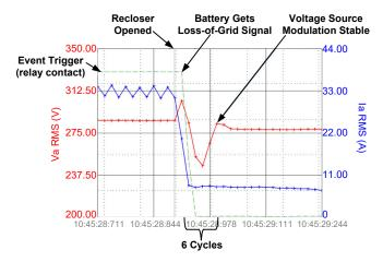
Fig. 1. Waveform of Transition From Grid-Connected to Island Mode
