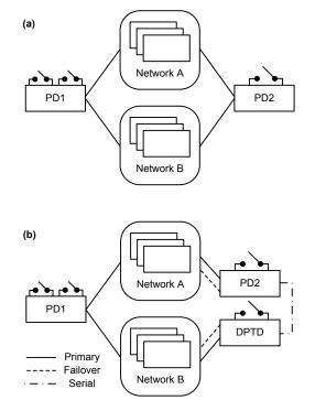
Fig. 6. Redundant Information Via Dual-Primary Contact Inputs (a) and Redundant Application Via a DPTD (b).
