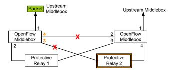
Fig. 12. OpenFlow Outputs Packet to Original Ingressing Port.
