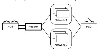
Fig. 8. Primary and Failover Cables, Singly Attached Node.
