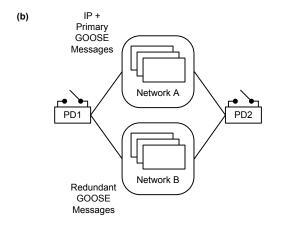
Fig. 5. Resilient Single Primary Ladder Network Topology (a) and Dual-Primary Signaling Via Two Systems Segregated by QVLANs (b).
