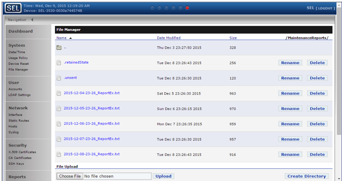
Figure 12 The RTAC Web Interface File Manager Menu Displaying Five Reports Generated Over a Five-Day Time Frame
