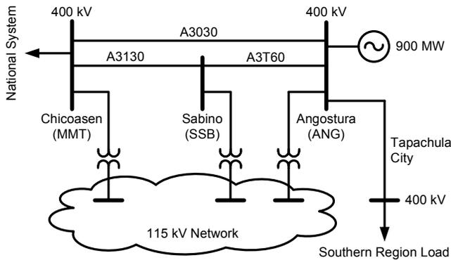
Fig. 11. Synchrophasor System One-Line Diagram
