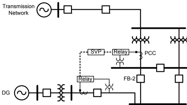
Fig. 8. DG One-Line Diagram for FPL
