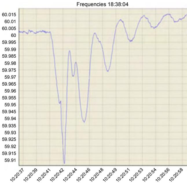
Fig. 7. Synchrophasor Data Plot Showing Frequency Excursion at Distribution Voltages
