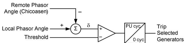
Fig. 12. Angle-Based AGSS Logic at Angostura
