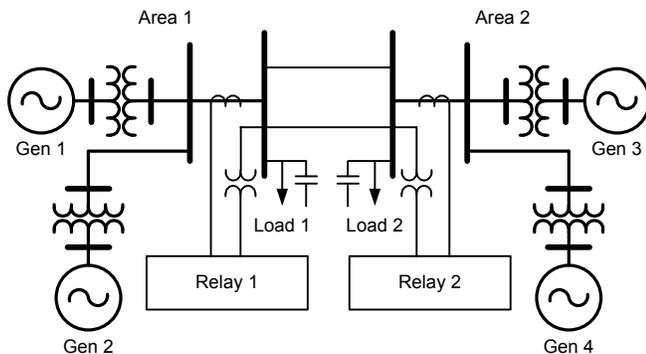
Fig. 15. Two-Area Power System Model With an Interarea Oscillation Problem
