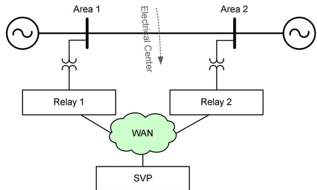
Fig. 13. Out-of-Step Detection System Configuration
