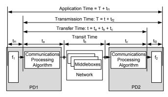
Fig. 1. Application, transmission, transfer, and transit time based on IEC  $61850\mathchar`-5$
