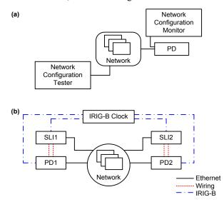
Fig. 2. Network configuration tester and monitor topologies (a) and test network (b)
