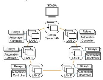
Fig. 4. Control center and multiple substation LANs connected in a ring
