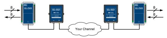
Figure 3 I/O Communications Including Secure Signal Encryption
