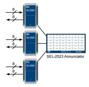
Figure 6 Bring in Remote I/O for Indication, Alarms, and Logic-Driven Remedial Actions
