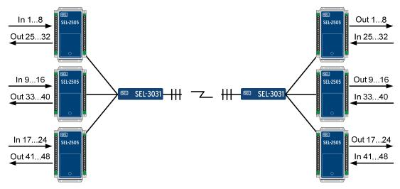
Figure 5 Three Serial Links of Information Can Transmit on a Single Radio
