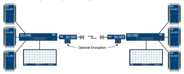
Figure 8 Mirrored Alarming at Remote Locations Provides Critical Information at Multiple Sites
