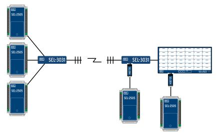
Figure 7 Radio Connection Provides Links to Contact I/O up to 20 Miles Away
