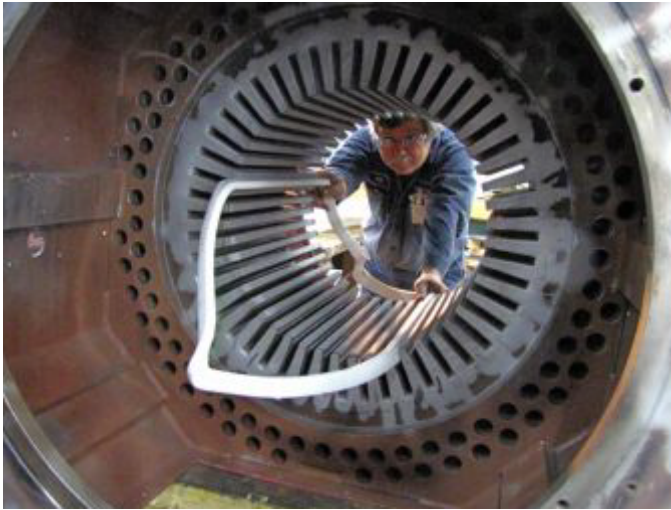
Fig. 4. Insertion of a Form-Wound Coil Winding Into a Small Synchronous Motor
