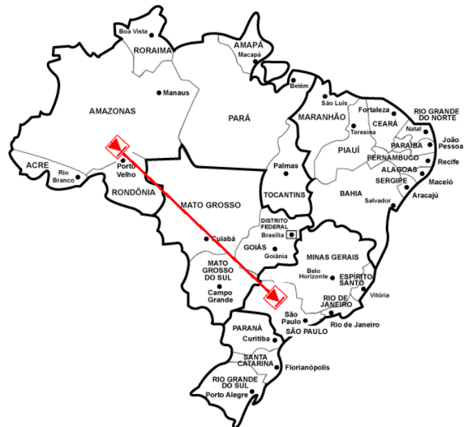
Fig. 1. 2,400 km bipolar 600 kV HVDC transmission lines connect the Porto Velho rectifier station and the Araraquara inverter station
