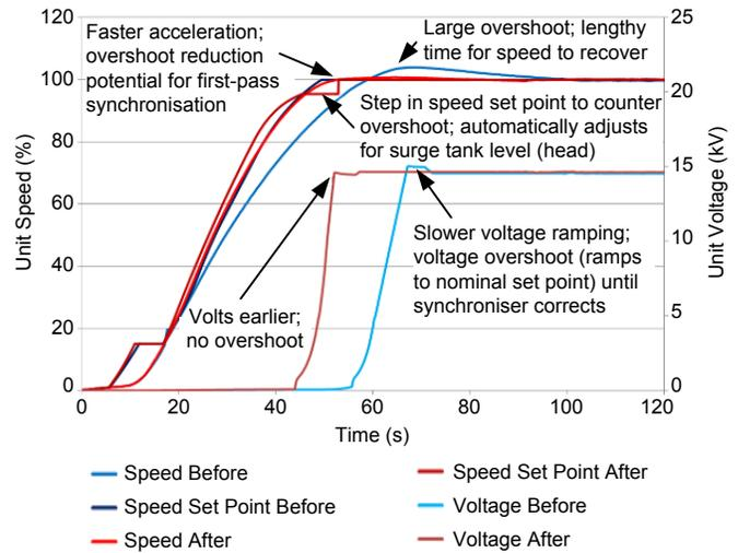
Fig. 16. Synchronising Time Reduction
