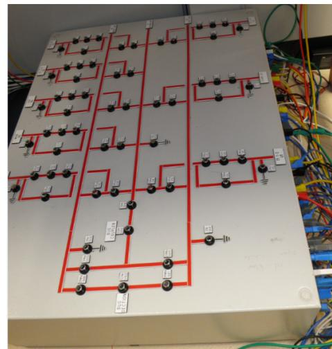
Fig. 13. Upper Tumut Switching Station Simulator for Testing
