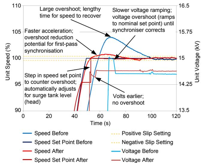
Fig. 17. Generator Speed Within Acceptable Synchronising Window
