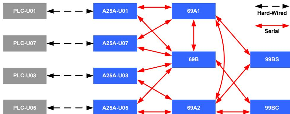
Fig. 4. Communications Diagram
