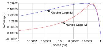
Fig. 8 Comparison of Single-Cage IM and Double-Cage IM Torque Versus Speed
