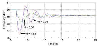
Fig. 1 Load Acceptance for Different Generator Inertias
