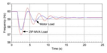
Fig. 2 Load Acceptance for Motor and ZIP-MVA Loads
