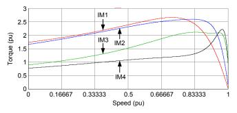
Fig. 6 IM Torque Versus Speed Characteristics
