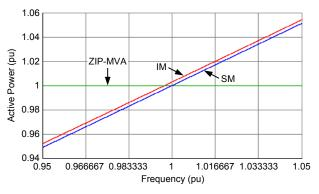
Fig. 11 Active Power Versus Frequency for SM, IM, and ZIP-MVA Loads
