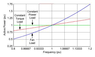
Fig. 10 Active Power Versus Frequency for Different Load Types
