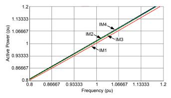
Fig. 7 Active Power Versus Frequency for Different IMs
