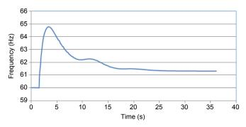
Fig. 3 Field Test Frequency Response for Load Rejection of 10.0 MW to 0 MW
