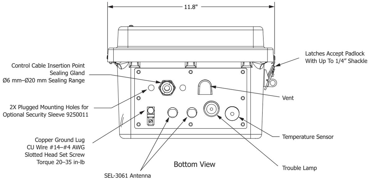
**Figure 2.5 Bottom View of Terminal Block Enclosure**
