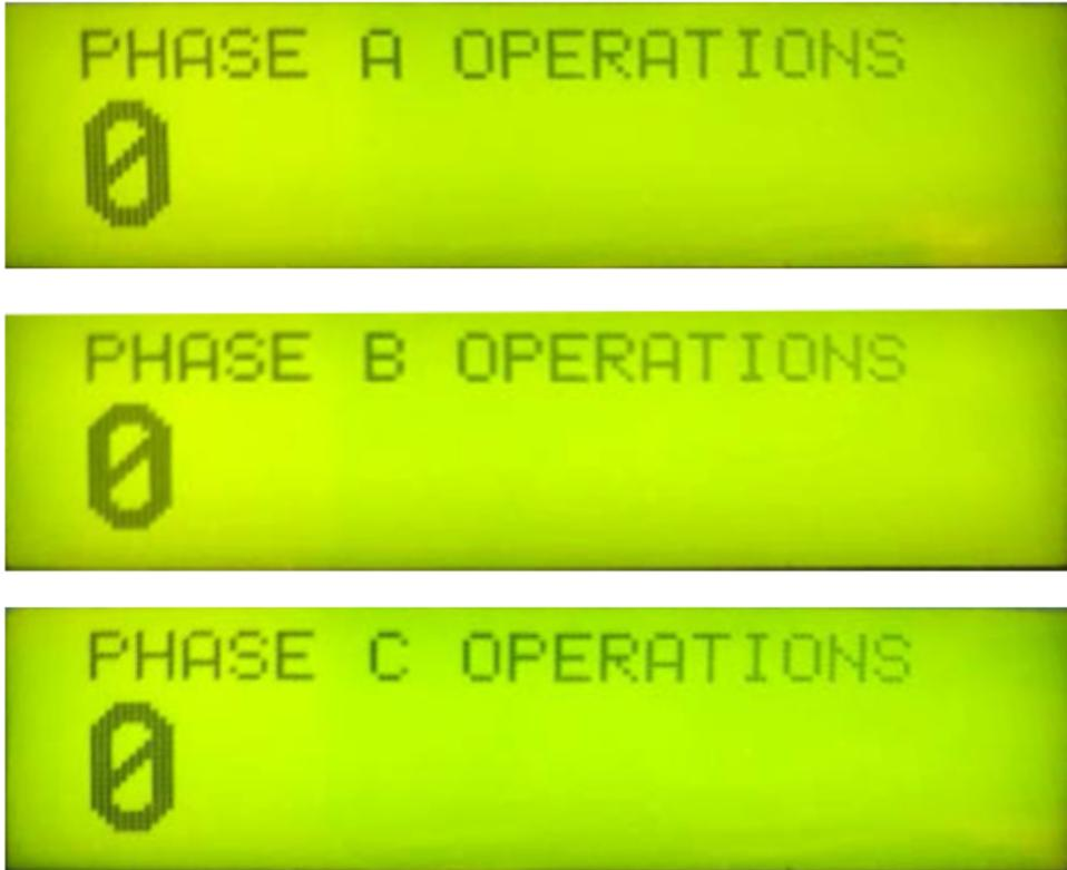
Figure 6.2 Operation Counters on the Rotating Front-Panel LCD
