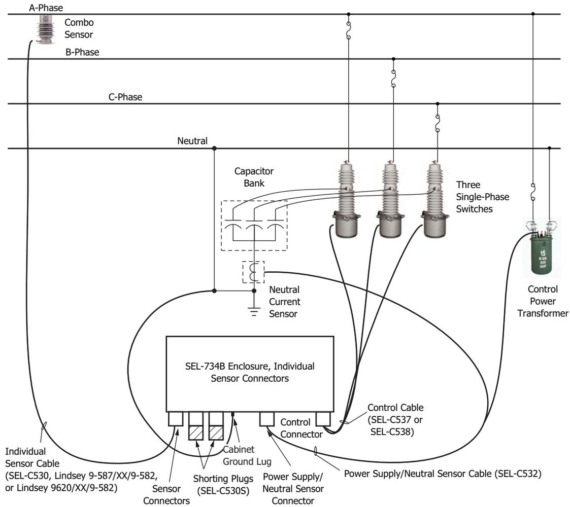
**Figure C.5 Full-Size Enclosure With Individual Sensor Connectors (Installed With a Single Combo Sensor and Generic Neutral Current Sensor)**
