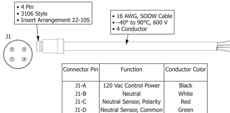
Power Supply/Neutral Sensor Cables for Full-Size Enclosures With Individual Sensor Connectors
