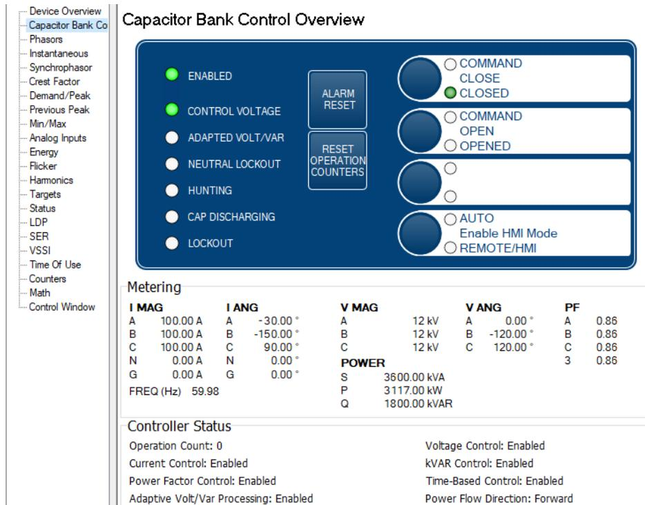
Figure 4.3 QuickSet HMI Capacitor Bank Control Overview
