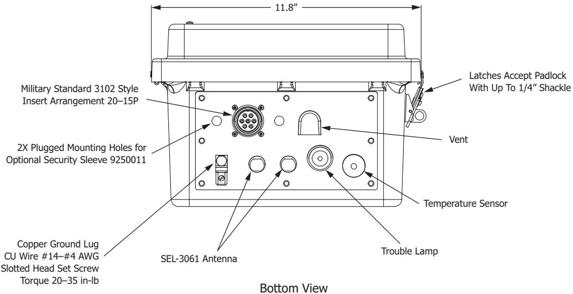
**Figure 2.4 Bottom View of Connectorized Compact Enclosure**
