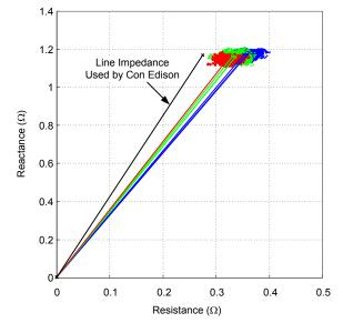
Fig. 14. Comparison of the Positive-Sequence Line Impedance Against the Line Impedance Used by Con Edison
