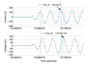
Fig. 16. Phase Voltages and Currents Captured at the Astoria Terminal During Cable Energization
