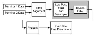
Fig. 10. Signal Processing to Compute Line Parameters
