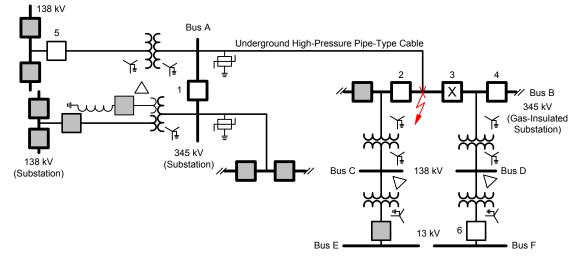
Fig. 1. System Used for Surge Arrester Energy Duty Analysis
