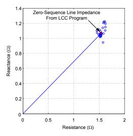
Fig. 12. Comparison of the Zero-Sequence Line Impedance Against the Line Parameters Reported by the LCC Program
