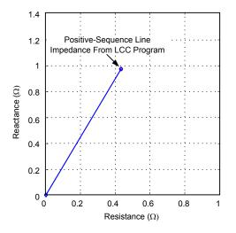
Fig. 11. Comparison of the Positive-Sequence Line Impedance Against the Line Parameters Reported by the LCC Program
