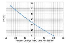
Fig. 3. GIC Flow Depends on the Line Resistance Accuracy
