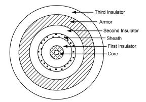
Fig. 4. Cross-Section of an Underground Cable
