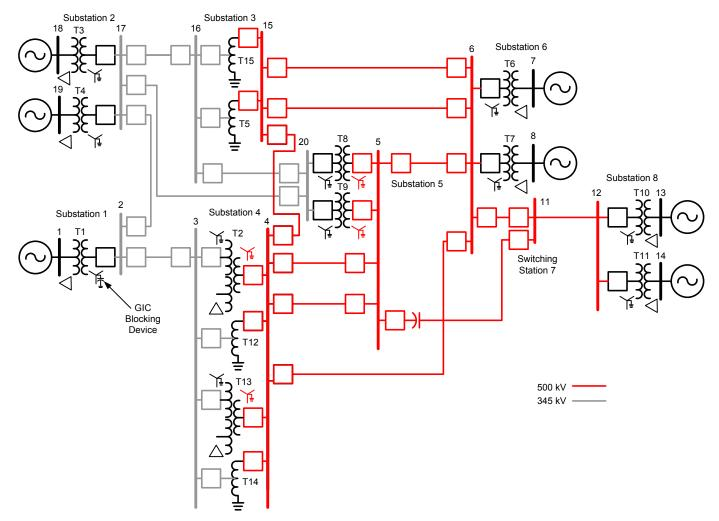
Fig. 2. System for GIC Flow Analysis
