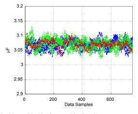
Fig. 15. Measured Positive-Sequence Line Capacitance
