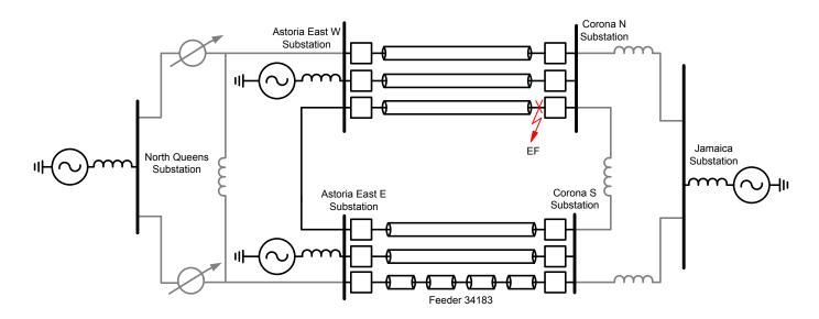
Fig. 9. System Diagram Showing Feeder 34183, the Cable Under Study; Transfer Impedances on Gray Lines Are Obtained From Network Reduction
