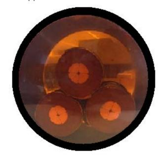
Fig. 8. Cables in a Close Triangular Configuration
