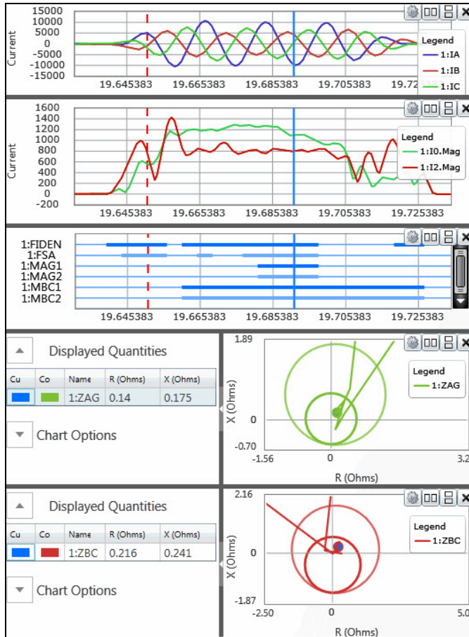
Fig. 11. Deerhaven Line 6 fault identification and impedance plots.
