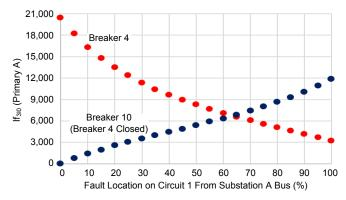
Fig. 2. Fault current variation seen by Breakers 4 and 10 for faults on Circuit 1
