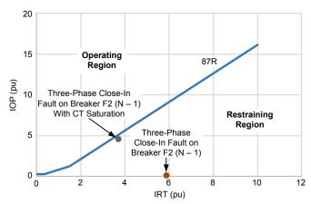
Fig. 10. Substation B bus differential characteristic and simulated external faults
