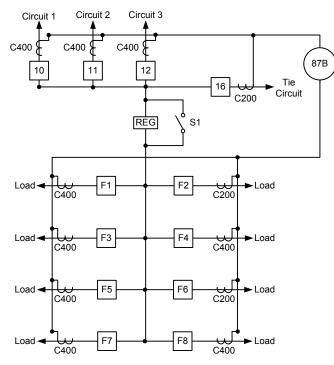
Fig. 6. Existing Substation B bus differential scheme CT connections
