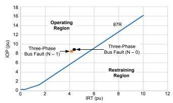
Fig. 9. Substation B bus differential characteristic and simulated internal (bus) faults
