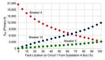
Fig. 3. Fault current variation as seen by Breakers 4, 5, and 10 for faults on Circuit 1  $\,$
