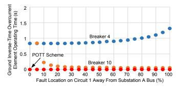
Fig. 13. POTT and ground inverse-time overcurrent element operating times as seen by Breakers 4 and 10 on Circuit 1
