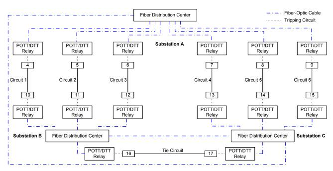
Fig. 11. Network communications layout for the POTT/DTT relay schemes
