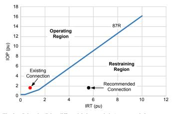
Fig. 8. Substation B bus differential characteristic (recommended versus existing connections)
