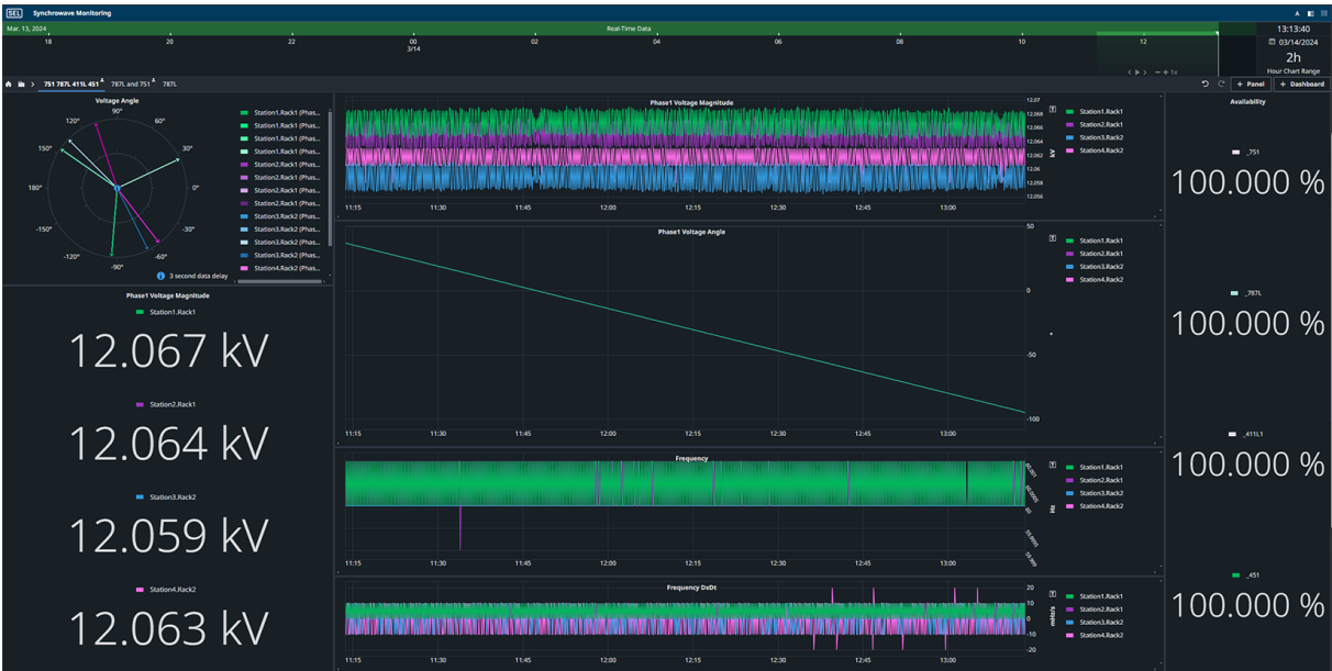
Figure 16 Visualization of Phase Angle Measurements Across a Power System
