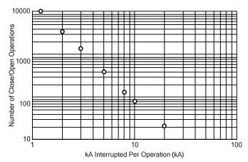
Fig. 3. Circuit breaker maintenance curve
