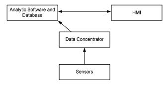
Fig. 1. Conventional monitoring system
