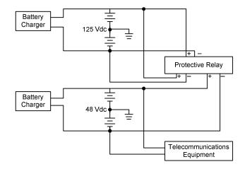
Fig. 6. Basic connection diagram for monitoring of two dc battery systems
