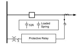
Fig. 4. Basic connection diagram for monitoring of circuit breakers
