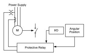
Fig. 11. Basic connection diagram for monitoring of disconnect switches
