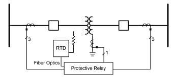
Fig. 8. Basic connection diagram for monitoring of transformers
