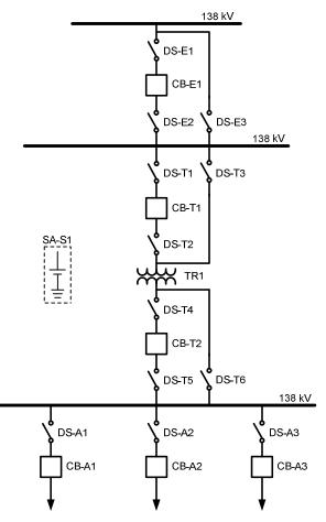
Fig. 14. One-line diagram of the simulation and test substation
