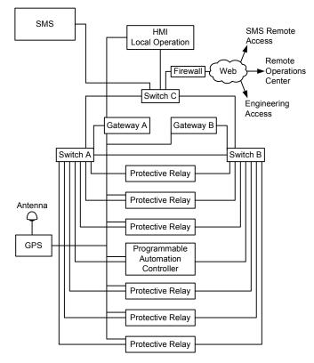
Fig. 13. Example of SMS integrated in the substation
